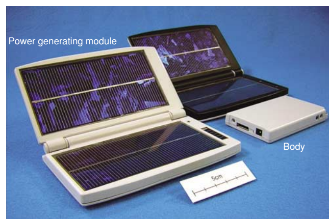
Solar-powered mobile power source (prototype)
