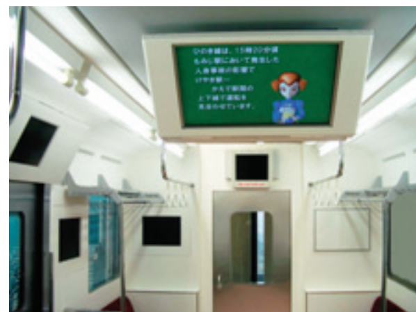
Simulated display of emergency messages via text and sign language inside a train
