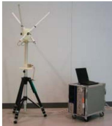
Radio field intensity measuring device with receiving antenna for measuring radio waves at mobile phone base stations
