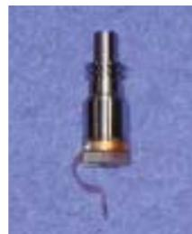
A module containing a laser chip developed by NTT Photonics Laboratories
