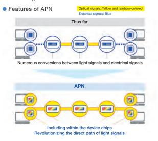
by converting all signals into optical signals, thereby creating a network with higher capacity, lower latency, and more reduced energy consumption than now.
