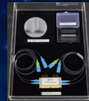
Quantum light source module developed by NTT
