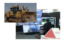
Remote operation of construction equipment, etc.
