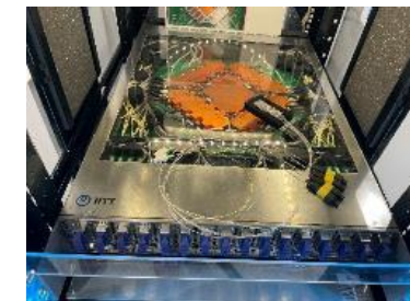
Prototype Switch with 51.2 Tbps Capacity
