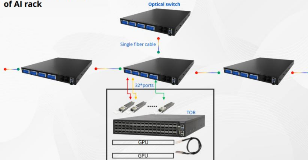
Optical switch on top of AI rack
