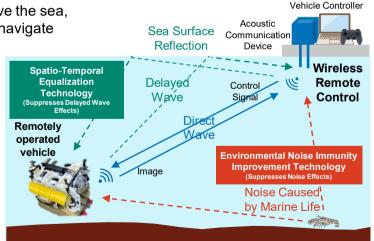
A technology that eliminates the degradation of communications quality caused by wave reflection from the sea surface, by eliminating part of the reflected waves in the spatial domain from the sea surface and seabed by using array technology that utilizes multiple wave receivers
