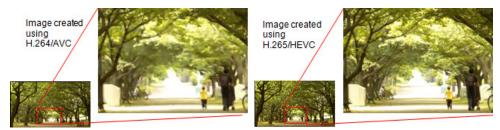
The two images are compared under the same conditions (bitrate: 2.5Mbps; frame rate: 29.97fps; and image size: 1080p). The image created by HEVC shows the tree leaves in finer detail.
